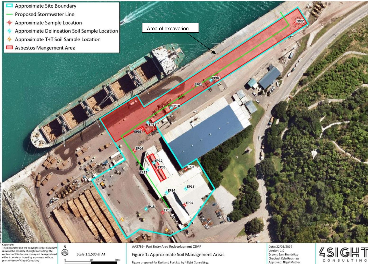
FIGURE 1: ASBESTOS MANAGEMENT AREA FROM 4SIGHT DETAILED SITE INVESTIGATION.
