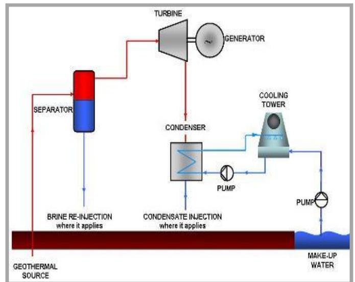
**Fig 2 - Condensing steam turbine process**
